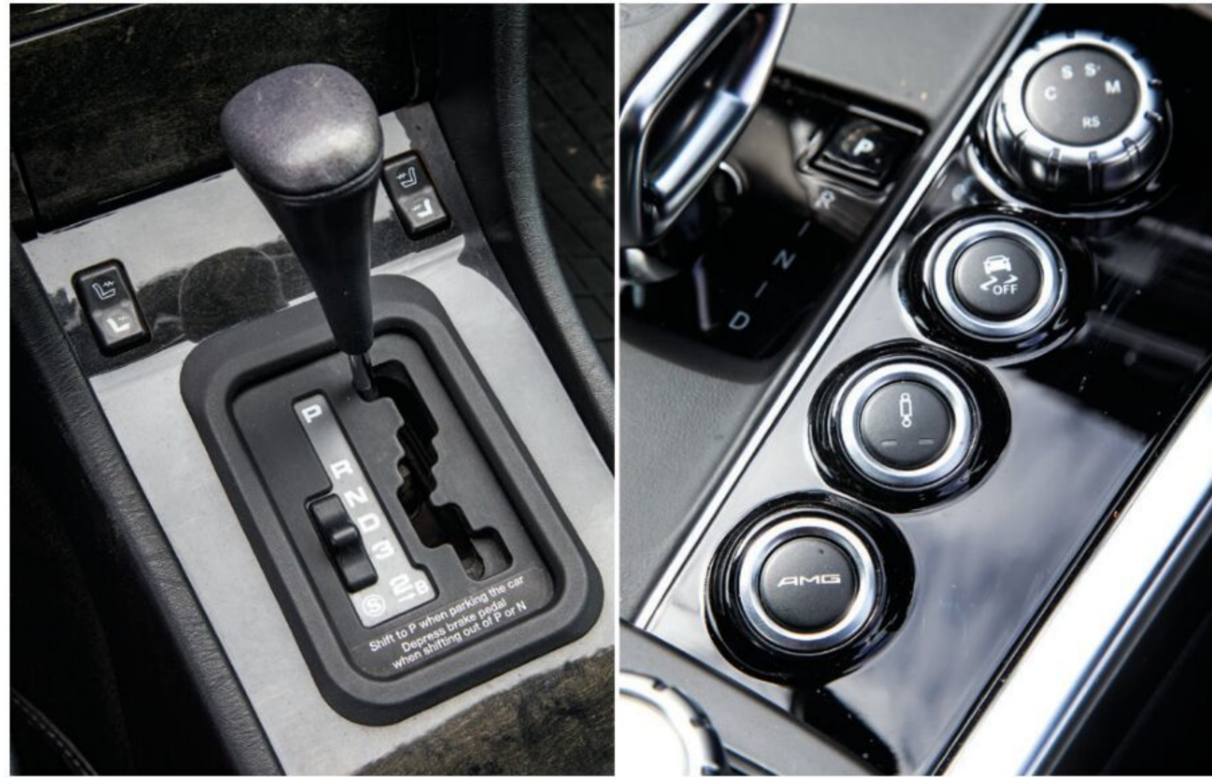
Far left Four gears and two modes for the W124 V8 car.
